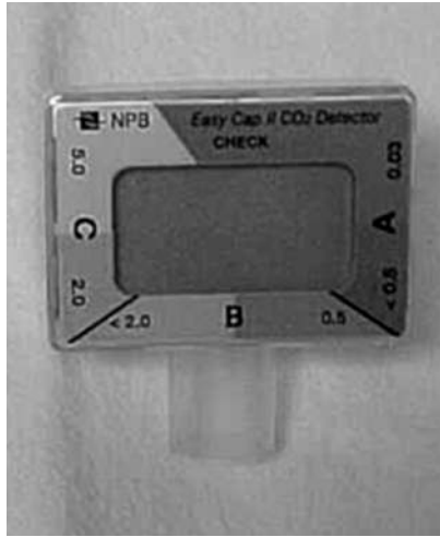
Figure 1-1. Colorimetric device. In infants and children with a perfusing rhythm, a purple color on the device indicates a problem, whereas a yellow color implies that the tube is in the trachea.
